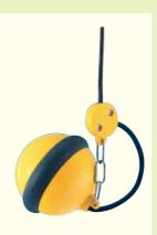
Model RF-5 is an economy type float which can detect upper/lower-limit water levels with single float. The snap onoff action ensures stable operation in clean or waste water containing suspended solids or oil and fat.
