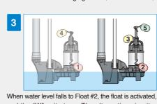
and the "W" unit stops. The alternating circuitry deactivates the "W" unit for the next level rise
