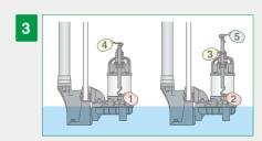
When water level falls and Float #1 is activated, the "A" unit stops. At the same time, "W" unit becomes ready for operation for the next level rise
