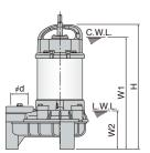
C.W.L.: Continuous Running Water Level L.W.L.: Lowest Running Water Level
